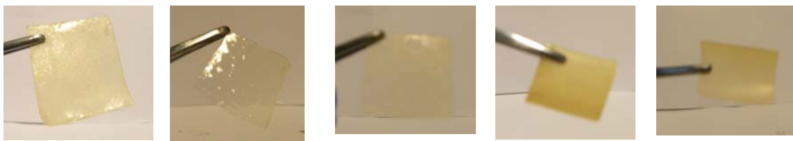
Figure 28. Appearance of Polymeric ionic liquid films as a function of %wt-cross-linker (from left to the right).
